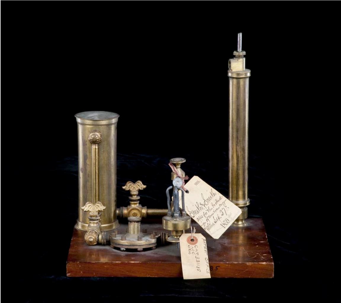
(Photo Courtesy Smithsonian Institution, National Museum of American History, Home and Community Life) RWS2012-04598 Patent 25611 Incandescent Gas Burner.
